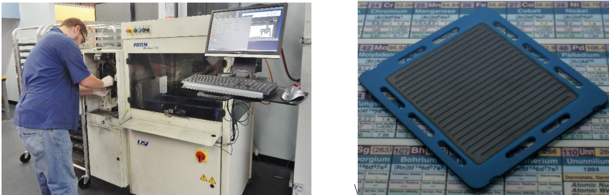
Figure 1. ChromLok™ coating process: (a) Nexceris facility for coating deposition (left); and (b) multi-compositional coating demonstrating spatial resolution and conformal coating of features (right).
