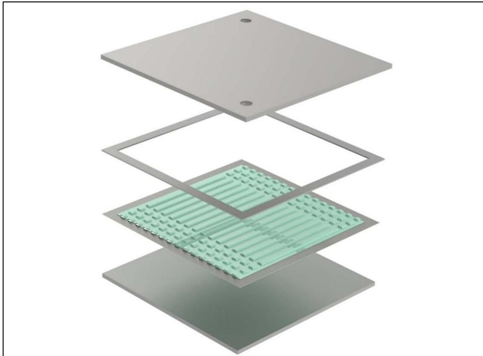
**Figure 4.** Rendered schematic of the catalyst-coated stainless-steel plate (441S, green color, 4.25"× 3.875"), in-between the Crofer 22APU manifold covers.
